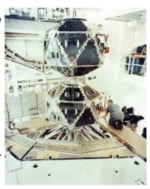
Vela 1, which refers to both satellites with the designations 1A and 1B, was launched atop an Atlas-Agena rocket on October 17, 1963, and put into a highly elliptical orbit which extended almost a third of the way to the moon. The two satellites were expected to last only about six months, but instead were operational for almost five years. The second set, Vela 2A and 2B, was launched on July 17, 1964, and the third, Vela 3A and 3B, on July 20, 1965.
